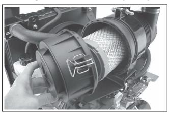
Figure 15. Removing End Cap.
